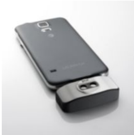
2015: FLIR One, an accessory to iPhone and Android mobile phones. Weight: 90 g (3.2 oz.).
