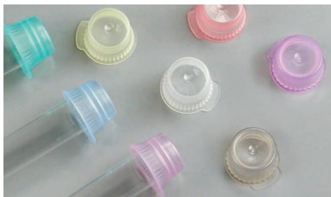
113139 (10mm) and 113142 (12mm) — Single tab series. Single thumb tab allows the tubes to be nested closely in test tube racks and still provides easy removal of the cap.
