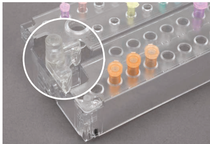
Locking tab allows multiple racks to be coupled to form a larger workstation.
